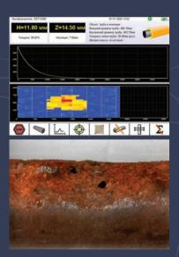
The measurement with the PE4332 instrument takes place on grid points. The user must apply a grid to the monitoring object before starting the diagnostic work. The user can draw a grid by hand using a ruler or stick a self-adhesive film on the pipe with a grid applied to it (our company supplies such a film). The measurement by the device takes place in the grid nodes, each measurement is displayed on the C-scan in the device.
