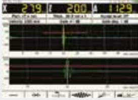
The signal can be represented in undetected form – **RF type signals** (radio signal) in real time, making it possible to examine signal phases in details, to perform testing with a lot of structural noises and to distinguish signals from nearby reflectors.
