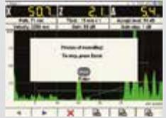
**Semiautomatic procedure of angle correction and delay time in the wedge in case of transducer wearing.**
