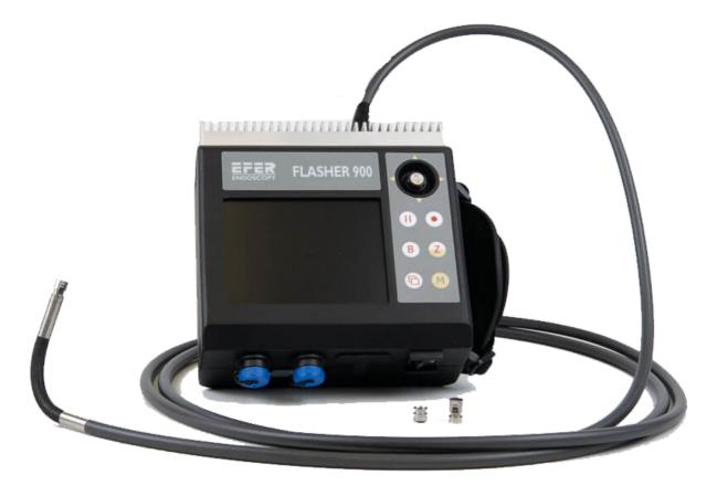
Portable expert probes with interchangeable distal tips, integrated image recording and joystick articulation control
