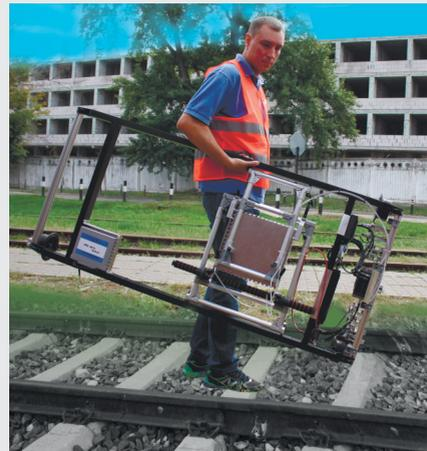
Weight of the assembled flaw detector does not exceed 22 kg.
