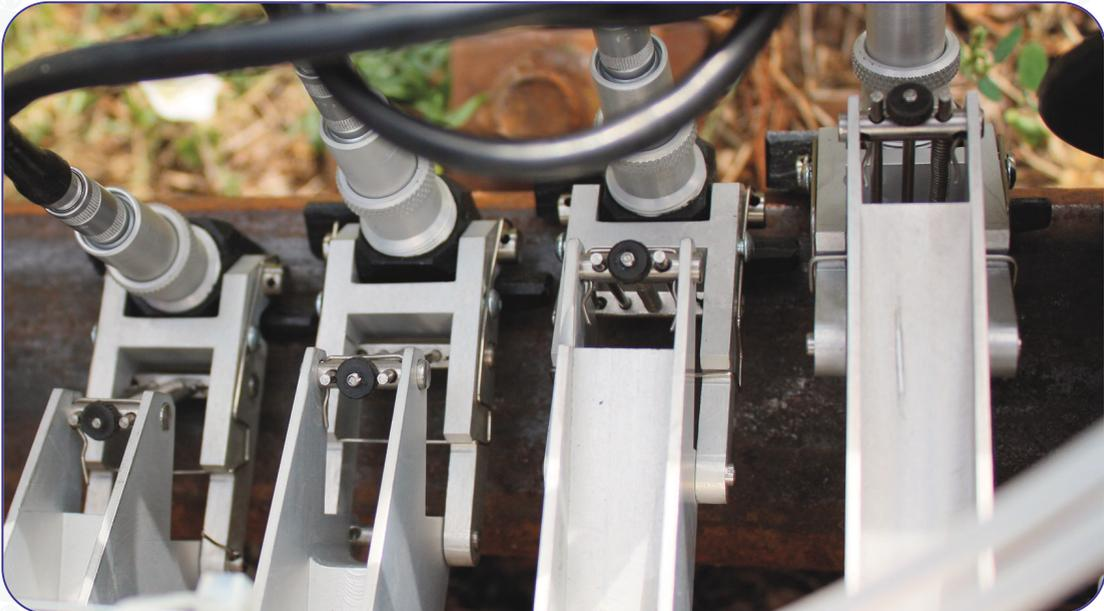
**The ETS2-77 flaw detector is a folding structure, which can be transported as it is assembled in stowed position**
