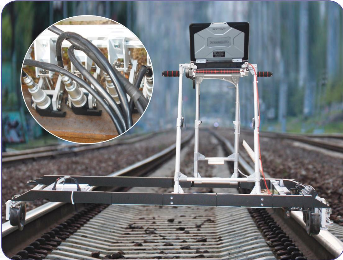
1 **ETS2-77** eddy current single rail flaw detector is a mechanized scanner which is intended for manual eddy current inspection of rail head's active face and running surface of rails laid down in a track, for the presence of surface cracks. The flaw detector serves for detection of flaws, e.g. cracks in the rail head, as well as for evaluation of their depth.
