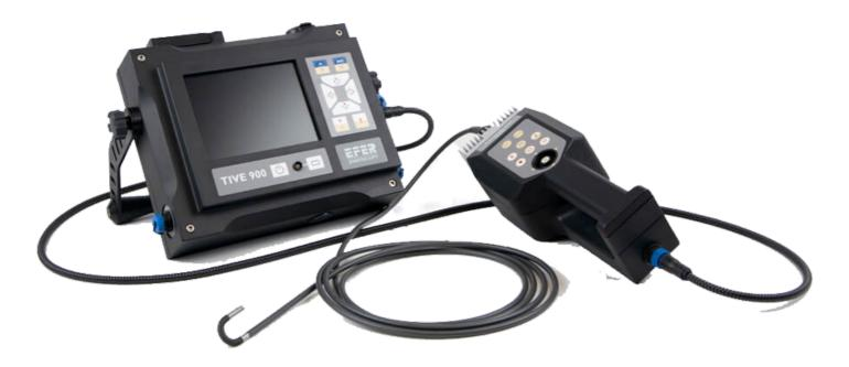
Expertise and measurement equipment comprised of an ARGUS 900 probe with operating unit.
